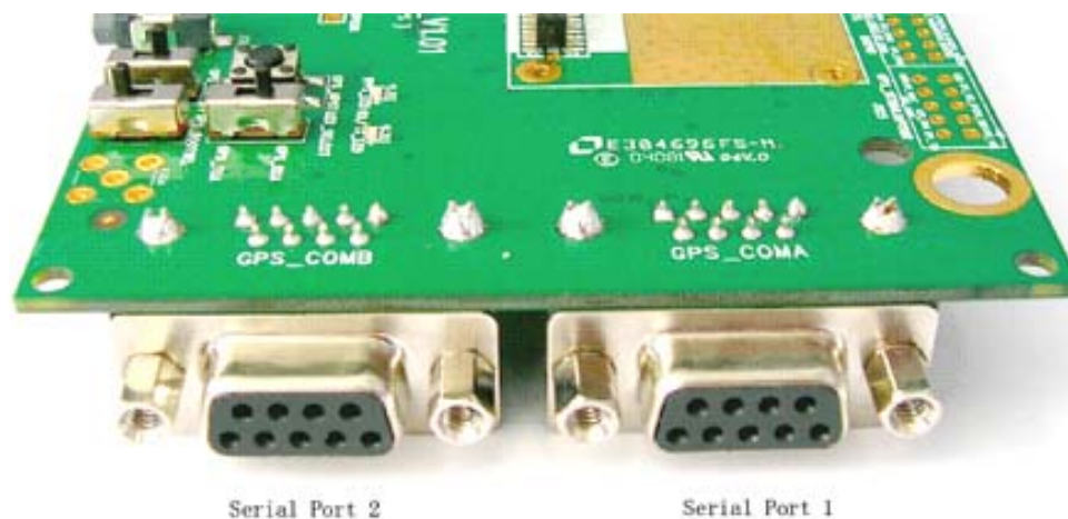
Figure 10: GPS part serial ports
