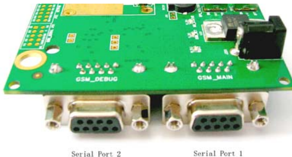
Figure 9: GSM part serial ports
