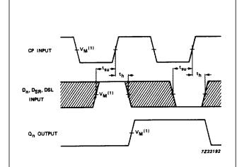
The shaded areas indicate when the input is permitted to change for predictable output performance.
