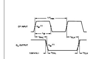
(1) HC :  $V_M$  = 50%;  $V_I$  = GND to  $V_{CC}$ . HCT:  $V_M$  = 1.3 V;  $V_I$  = GND to 3 V.
