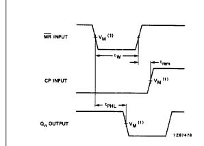
(1) HC :  $V_M$  = 50%;  $V_I$  = GND to  $V_{CC}$ . HCT:  $V_M$  = 1.3 V;  $V_I$  = GND to 3 V.
