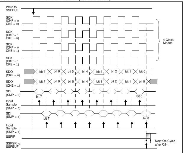
FIGURE 17-3: SPI MODE WAVEFORM (MASTER MODE)
