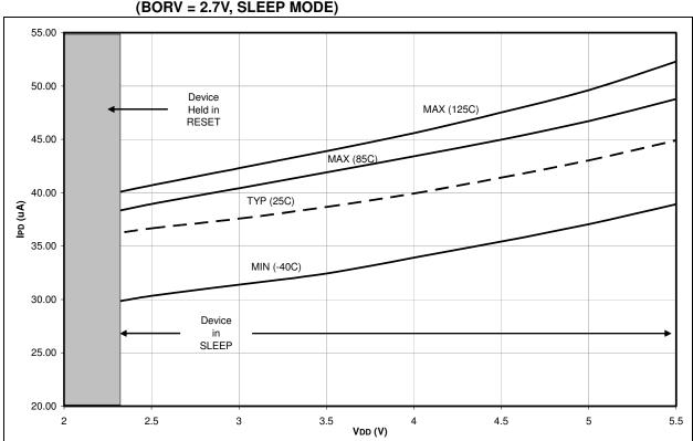
FIGURE 27-8: TYPICAL BOR DELTA CURRENT vs. VDD ACROSS TEMP. (BORV = 2.7V, SLEEP MODE)
