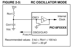
The RCIO Oscillator mode (Figure 2-6) functions like the RC mode, except that the OSC2 pin becomes an additional general purpose I/O pin. The I/O pin becomes bit 6 of PORTA (RA6).
