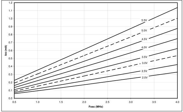
FIGURE 27-25: TYPICAL IDD vs. Fosc, 500 kHz TO 4 MHz (PRI\_IDLE MODE, 25 ℃)
