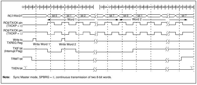
FIGURE 18-11: SYNCHRONOUS TRANSMISSION
