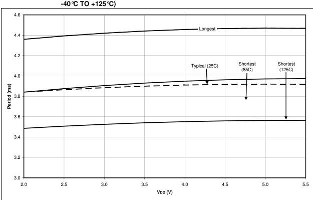
FIGURE 27-39: WDT PERIOD vs. VDD ACROSS TEMPERATURE (1:1 POSTSCALER, -40 ℃ TO +125 ℃)
