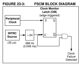
Clock failure is tested for on the falling edge of the sample clock. If a sample clock falling edge occurs while CM is still set, a clock failure has been detected (Figure 23-4). This causes the following:
