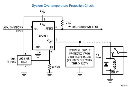
LM34 for 125 F Shutdown LM35 for 125 C Shutdown
