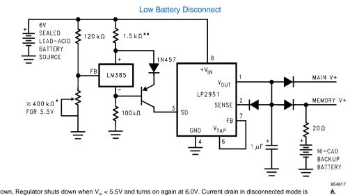
For values shown, Regulator shuts down when V<sub>in</sub> < 5.5V and turns on again at 6.0V. Current drain in disconnected mode is \*Sets disconnect Voltage
