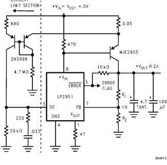
$V_{out} = 1.23V \left(1 + \frac{R_1}{R_2}\right)$
