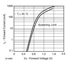
Figure 2. Forward Current vs. Forward Voltage
