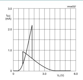
Fig 13. Typical 74HCT1G14 transfer characteristics;  $V_{CC} = 5.5 \text{ V}$
