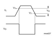
Fig 8. The definitions of V<sub>T+</sub>, V<sub>T-</sub> and V<sub>H</sub>; where V<sub>T+</sub> and V<sub>T-</sub> are between limits of 20 % and 70 %
