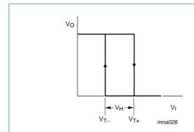
Fig 7. Transfer characteristic
