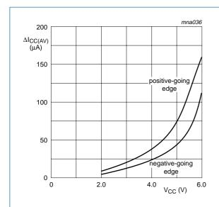
Fig 14.  $\Delta I_{CC(AV)}$  for 74HC1G14 devices; linear change of  $V_1$  between  $0.1 \times V_{CC}$  to  $0.9 \times V_{CC}$
