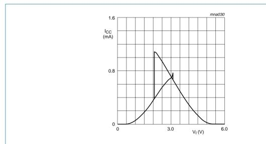
Fig 11. Typical 74HC1G14 transfer characteristics; V<sub>CC</sub> = 6.0 V
