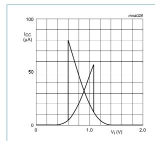
Fig 9. Typical 74HC1G14 transfer characteristics;  $V_{CC} = 2.0 \text{ V}$
