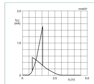
Fig 12. Typical 74HCT1G14 transfer characteristics;  $V_{CC} = 4.5 \text{ V}$
