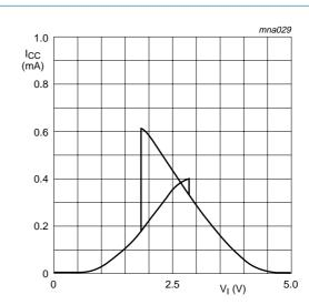
Fig 10. Typical 74HC1G14 transfer characteristics;  $V_{CC} = 4.5 \text{ V}$
