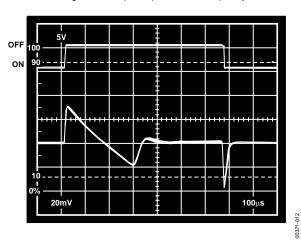
Figure 12. Load Transient Response
