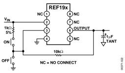
Figure 22. Membrane Switch Controlled Power Supply
