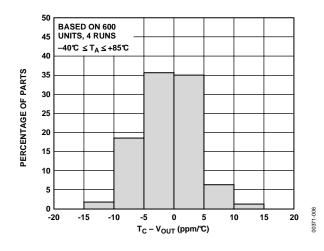
Figure 6.  $T_C - V_{OUT}$  Distribution
