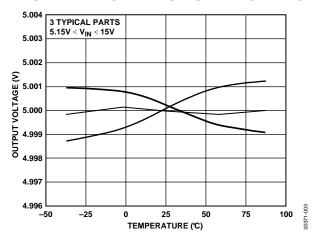
Figure 3. REF195 Output Voltage vs. Temperature
