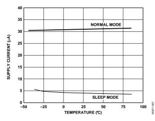
Figure 7. Supply Current vs. Temperature
