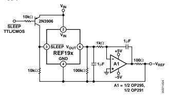
Figure 24. Negative Precision Voltage Reference Uses No Precision Resistors
