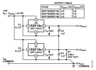
Figure 25. Stacking Voltage References with the REF19x
