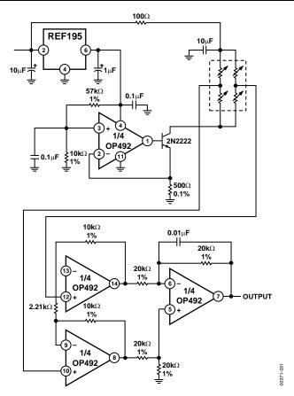
Figure 31. A Low Power, Strain Gage Circuit
