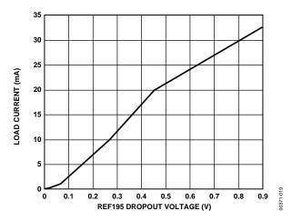
Figure 19. Load Current vs. Dropout Voltage
