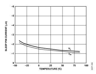
Figure 8. SLEEP Pin Current vs. Temperature
