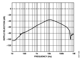
Figure 9. Ripple Rejection vs. Frequency
