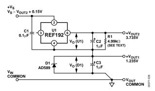
Figure 26. Stacking Voltage References with the REF192
