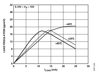
Figure 4. REF195 Load Regulator vs. ILOAD
