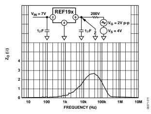
Figure 11. Output Impedance vs. Frequency
