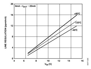
Figure 5. REF195 Line Regulator vs. V<sub>IN</sub>
