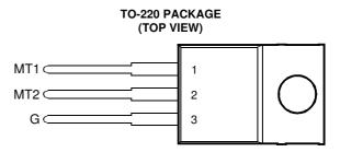
Pin 2 is in electrical contact with the mounting base.
