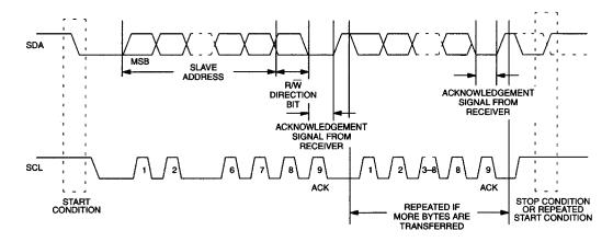
Figure 6 details how data transfer is accomplished on the two-wire bus. Depending upon the state of the  $R/\overline{W}$  bit, two types of data transfer are possible:
