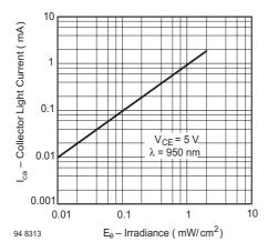
Figure 4. Collector Light Current vs. Irradiance
