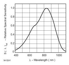
Figure 8. Relative Spectral Sensitivity vs. Wavelength
