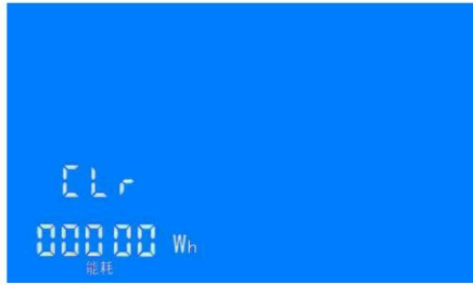
Figure 9 clear the energy interface
