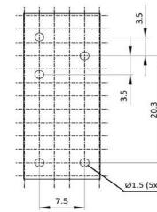
**RT78602**, Socket with PCB terminals, pinning 5 mm
