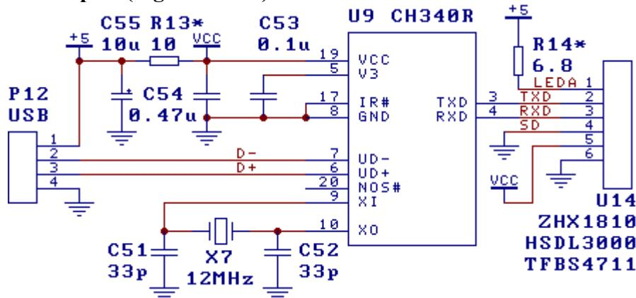
The figure above is a USB infrared adapter composed of USB to IrDA infrared chip CH340R and infrared transceiver U14 (ZHX1810/HSDL3000 and other similar models). Resistor R13 is used to weaken the impact of large current on other circuits during the infrared transmission process, and can be removed when the requirements are not high. The current limiting resistor R14 should be adjusted according to the recommended value of the manufacturer of the actually selected infrared transceiver U14.
