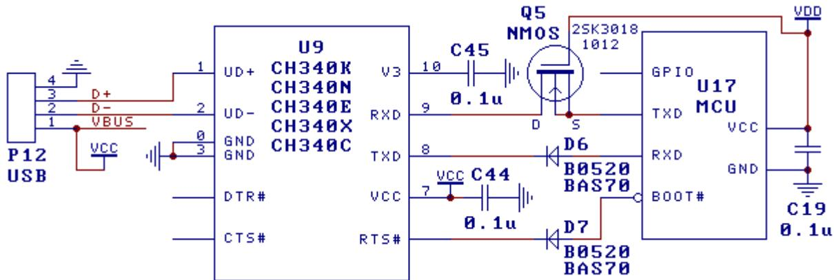
The figure above is a reference circuit for connecting the MCU microcontroller to the CH340 chip through the TTL serial port to achieve USB communication in dual power supply mode. CH340 is powered by the USB bus VBUS, and the MCU uses another power supply VDD. VDD supports 5V, 3.3V or even 2.5V and 1.8V.
