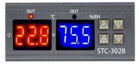
Long press  $\triangle$  3 seconds, the starting temperature value flashes (default 20 ° C) Press the plus or minus button to adjust, long press  $\nabla$  3 seconds, stop the temperature value flash (default 30 ° C) press the plus or minus button to adjust.
