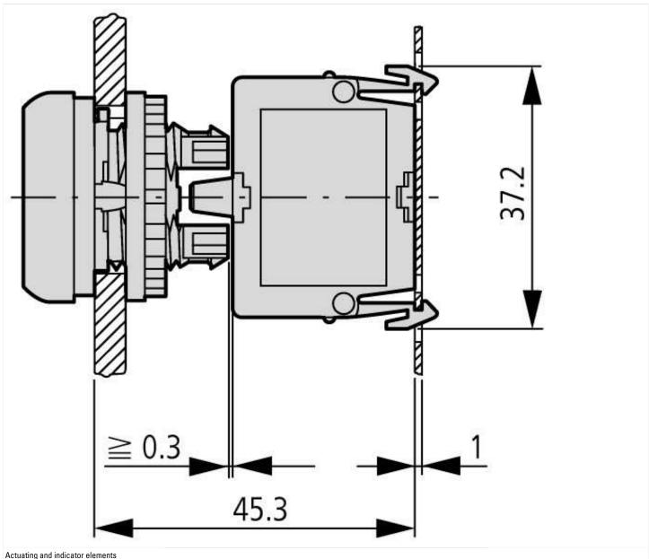
Actuating and indicator elements Base fixing
