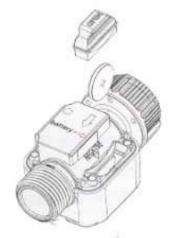
Step 2: Install the battery and let the battery positive face outward.
