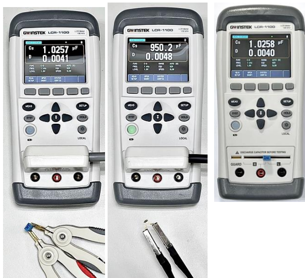
Figure Test results for capacitors
