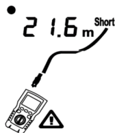
Figure 6.16 Short on Coaxial Cabling
