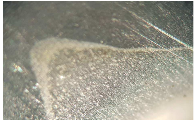
Results: Aluminium corrosion
