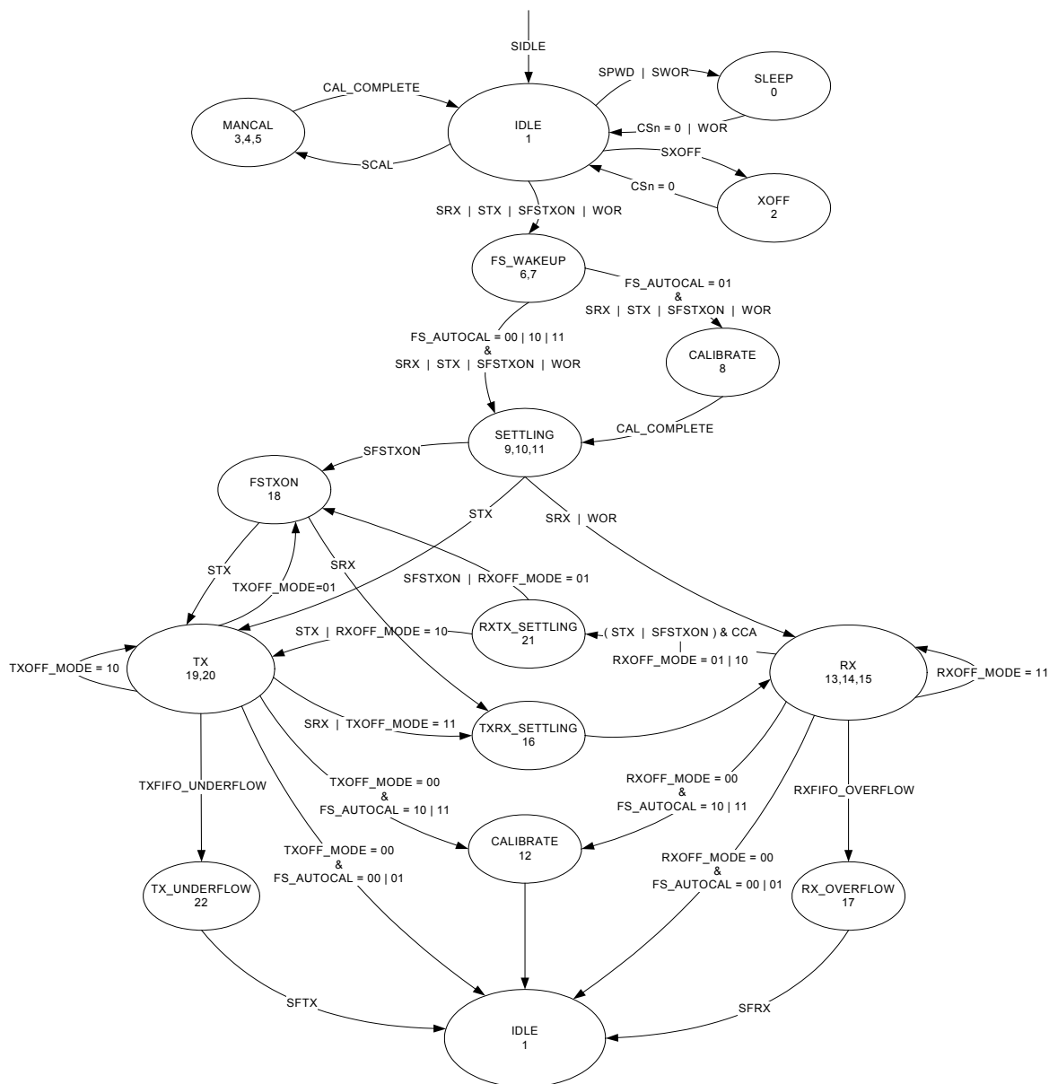
Figure 16: Complete Radio Control State Diagram
