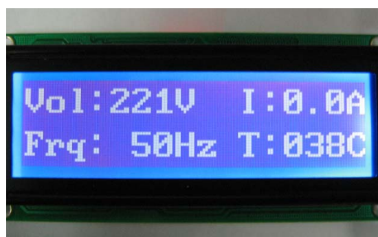
Figure 3-2. Connection between EGS002 and 12832 LCD Figure 3-3. 12832 LCD Display
