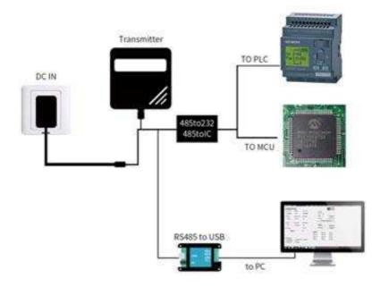
This product can also be used by multiple sensors combined in a 485 bus. In theory, one bus can connect more than 16 485 sensors. If more 485 sensors are needed, more 485 devices can be expanded using 485 repeaters. The other end is
