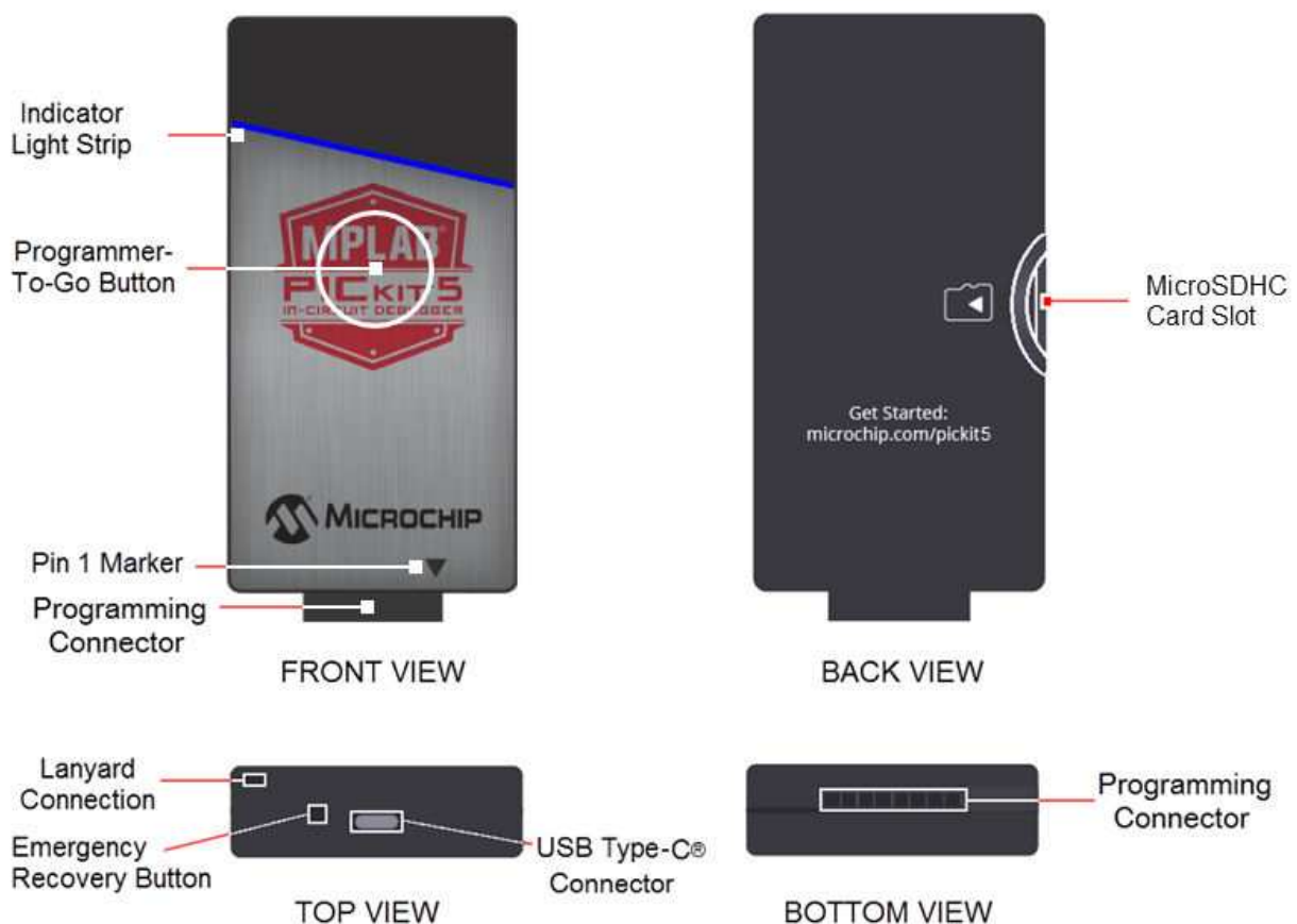
Figure 5-1. MPLAB® PICKit™ 5 In-Circuit Debugger Diagram
