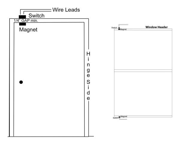
Surface mount switch at top or side (NOT on hinge side) of door or hinged window frame On double hung window, surface mount the switch at top, side or bottom of window frame Surface mount the magnet parallel to the switch
