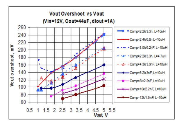
Figure 3. Load Transient Testing VS Compensation Value
