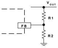
Figure1. Output Voltage Setting
