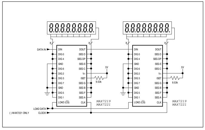
Figure 3. Cascading MAX7219/MAX7221s to Drive 16 7-Segment LED Digits
