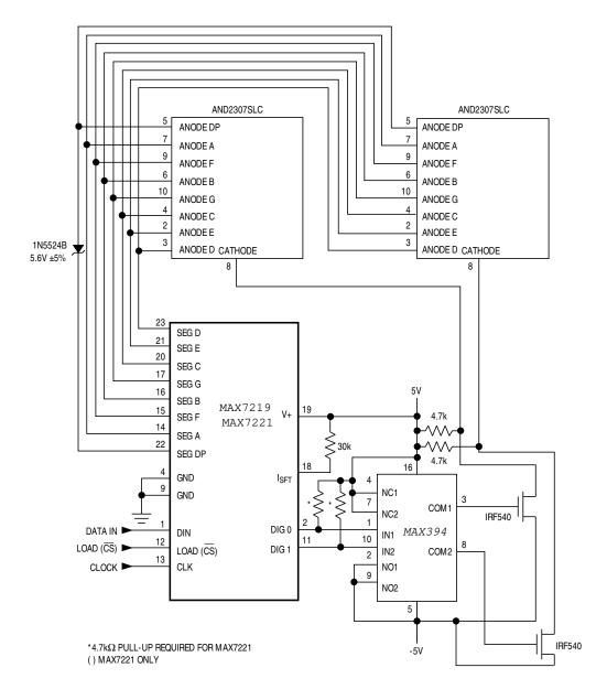
Figure 2. MAX7219/MAX7221 Driving 2.3-Inch Displays
