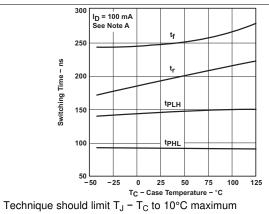
Figure 5. Switching Time vs Case Temperature
