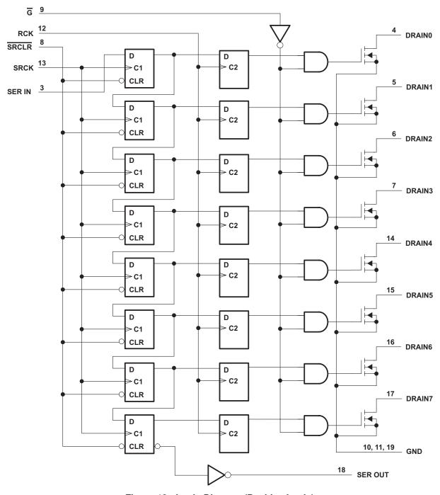
Figure 12. Logic Diagram (Positive Logic)
