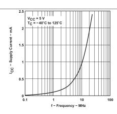
Figure 2. Supply Current vs Frequency
