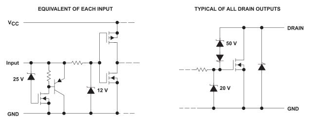
Figure 13. Schematic of Inputs
