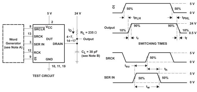
INPUT SETUP AND HOLD WAVEFORMS
