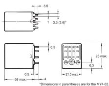
PCB Processing Dimensions (Bottom View)
