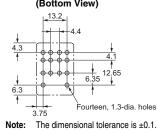
**Terminal Arrangement/Internal** Connections (Bottom View) Standard Models
