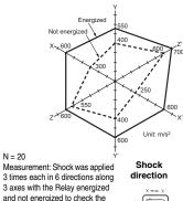
and not energized to check the shock values that cause the Relay to malfunction. Criteria: Non-energized: 200 m/s<sup>2</sup> Energized: 200 m/s<sup>2</sup>
