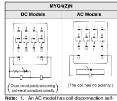
diagnosis 2. For the DC models, check the coil polarity when wiring and wire all connections correctly.
