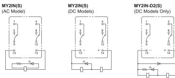
Note: For the DC models, check the coil polarity when wiring and wire all connections correctly.
