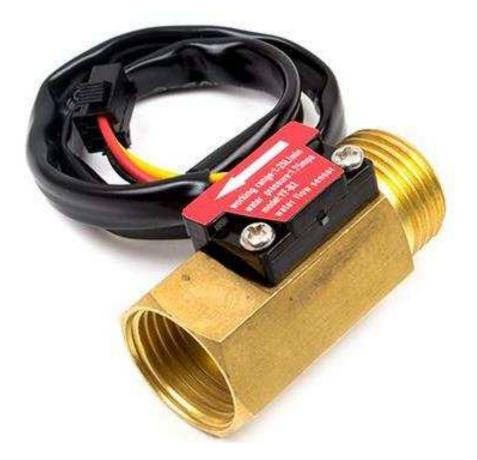
It consists of a copper body, a water rotor, and a hall-effect sensor. When water flows through the rotor, rotor rolls. Its speed changes with different rate of flow. The hall-effect sensor outputs the corresponding pulse signal.
