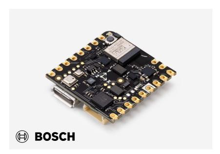
Featuring a 9DoF smart motion sensor and a multi parametric environmental sensor with AI capabilities, the board developed with Bosch Sensortec allows for a wide range of **IoT applications**. Having Arduino's signature simplicity of integration and scalability, it is also perfect for **research projects**, **rapid prototyping and development**.
