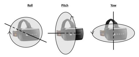
Figure 1: Headset Rotation Axes
