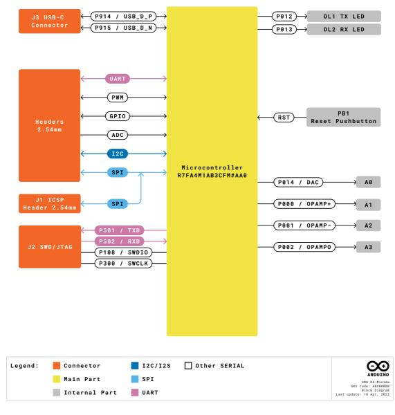
Arduino R4 Minima Block Diagram
