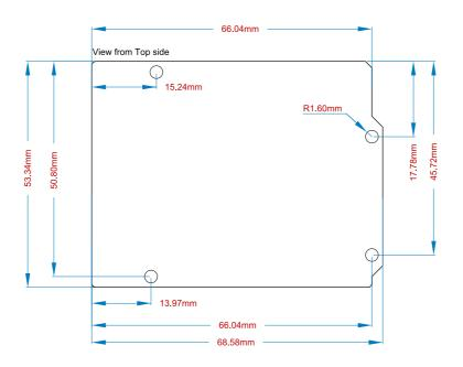
Mechanical View of Arduino UNO R4 Minima
