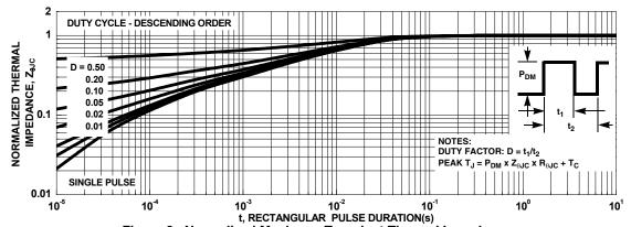
Figure 3. Normalized Maximum Transient Thermal Impedance
