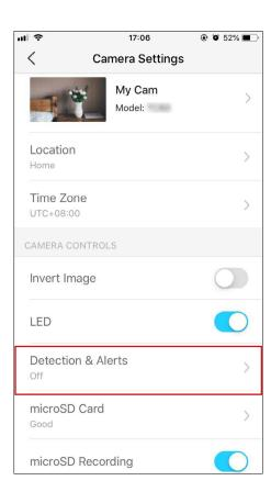
2. On the Detection & Alerts page, enable the Motion Detection function. It's recommended to enable the Notifications function to receive motion detection messages.
