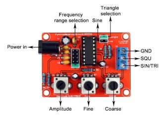
X2206 monolithic integration function generator generates high quality, high stability, high precision sine wave, square wave and triangular wave, can realize frequency modulation and amplitude modulation, suitable for circuits such as waveform generation, Scan production, AM/FM generation, FSK generation, and a phase-locked loop.
