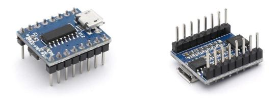
The module contains an MP3 chip that provides a serial port and perfectly integrates hardware decoding of MP3 and WAV. At the same time, the software supports SD card drive, supports direct update of SPI flash content via computer, and supports FAT16, FAT32 file systems. Functions such as playing specified music can be performed with a simple serial port command without the need for cumbersome underlying operations.
