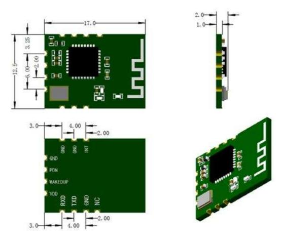
Fig4. Module Size Diagram
