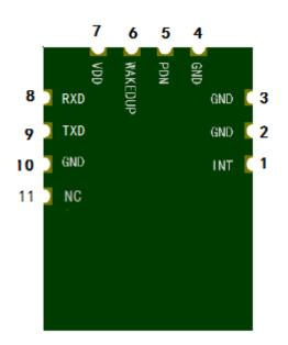
Fig. 3. Module Pins Distribution Diagram (Bottom View)
