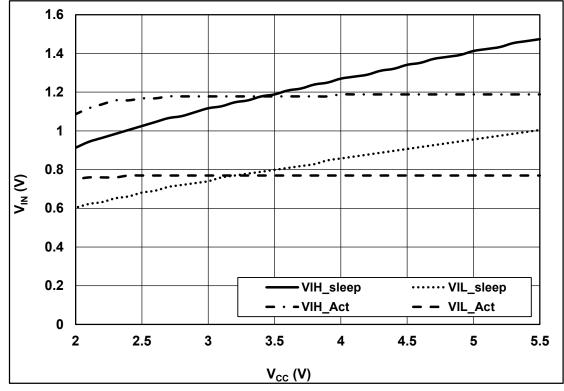
When a common voltage is used for the ATECC608A  $V_{CC}$  pin and the input pull-up resistor, then the TTLenable bit should be set to a one, which permits the input thresholds to track the supply as shown in Figure 2-5.
