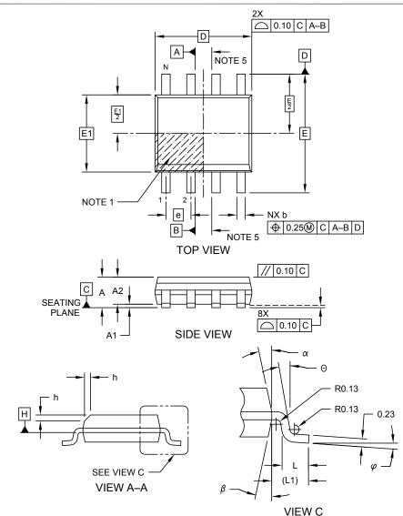
Microchip Technology Drawing No. C04-057-Atmel Rev D Sheet 1 of 2
