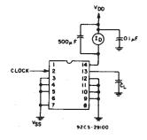
Fig. 14 - Dynamic power dissipation test circuit.
