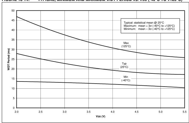
FIGURE 18-15: AVERAGE WDT PERIOD vs. VDD OVER TEMPERATURE (-40°C TO +125°C)
