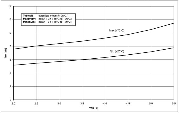
FIGURE 18-12: TYPICAL AND MAXIMUM AIWDT vs. VDD OVER TEMPERATURE (WDT ENABLED)
