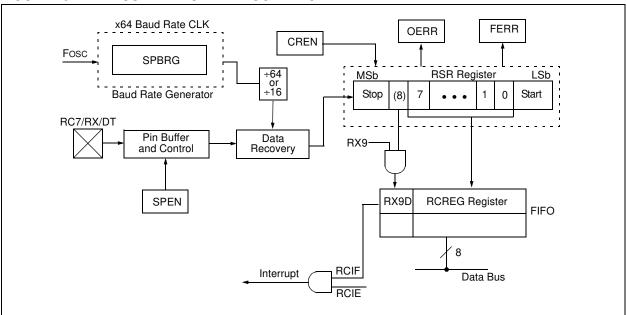
FIGURE 10-5: ASYNCHRONOUS RECEPTION
