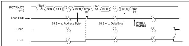
**Note:** This timing diagram shows a data byte followed by an address byte. The data byte is not read into the RCREG (Receive Buffer) because ADDEN was not updated and still = 0.
