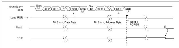
Note: This timing diagram shows a data byte followed by an address byte. The data byte is not read into the RCREG (Receive Buffer) because ADDEN = 1.
