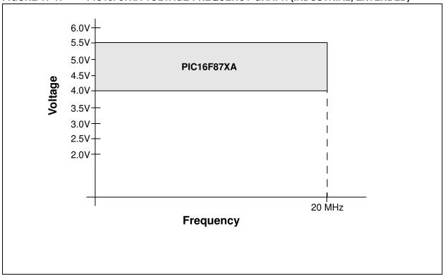
FIGURE 17-2: PIC16LF87XA VOLTAGE-FREQUENCY GRAPH (INDUSTRIAL)
