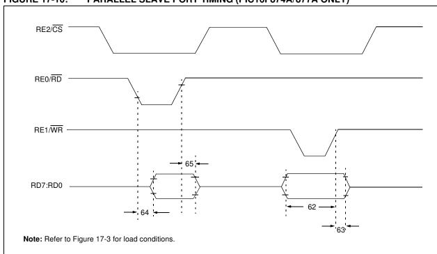
FIGURE 17-10: PARALLEL SLAVE PORT TIMING (PIC16F874A/877A ONLY)
