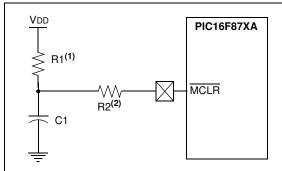
Note 1: R1 < 40 k $\Omega$  is recommended to make sure that the voltage drop across R does not violate the device's electrical specification.
