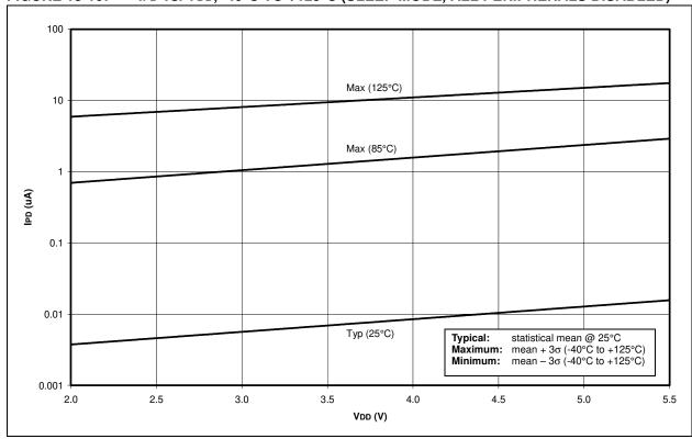
FIGURE 18-11: TYPICAL AND MAXIMUM  $\triangle$ ITMR1 vs. VDD OVER TEMPERATURE (-10°C TO +70°C, TIMER1 WITH OSCILLATOR, XTAL = 32 kHz, C1 AND C2 = 47 pF)
