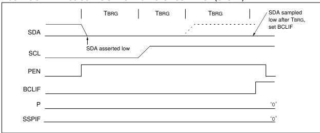
FIGURE 9-32: BUS COLLISION DURING A STOP CONDITION (CASE 2)
