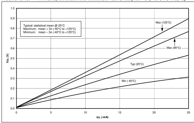
FIGURE 18-19: TYPICAL, MINIMUM AND MAXIMUM Vol vs. lol (VDD = 3V, -40°C TO +125°C)
