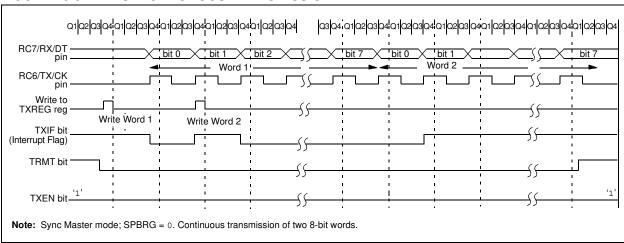
FIGURE 10-10: SYNCHRONOUS TRANSMISSION (THROUGH TXEN)
