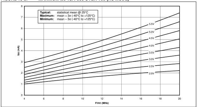
FIGURE 18-3: TYPICAL IDD vs. Fosc OVER VDD (XT MODE)
