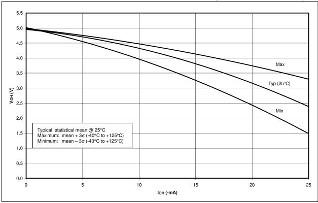
FIGURE 18-17: TYPICAL, MINIMUM AND MAXIMUM VOH vs. IOH (VDD = 3V, -40°C TO +125°C)
