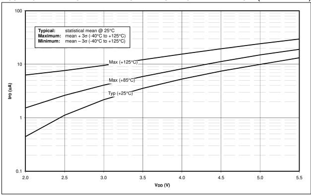
FIGURE 18-13: △IBOR vs. VDD OVER TEMPERATURE
