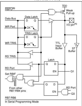
Note 1: I/O pins have diode protection to VDD and Vss.
