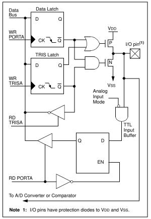
FIGURE 4-2: BLOCK DIAGRAM OF RA4/T0CKI PIN
