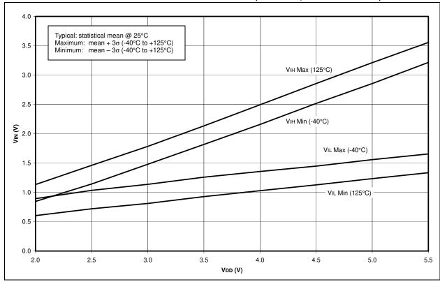
FIGURE 18-22: MINIMUM AND MAXIMUM VIN vs. VDD (I<sup>2</sup>C INPUT, -40°C TO +125°C)
