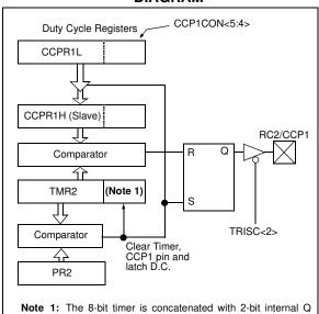
A PWM output (Figure 8-4) has a time base (period) and a time that the output stays high (duty cycle). The frequency of the PWM is the inverse of the period (1/period).
