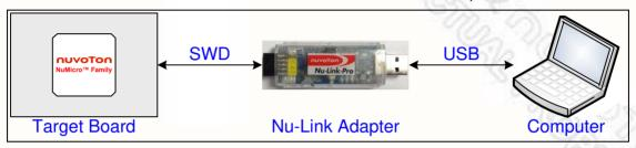
Figure 4-1 Nu-Link Adapter Connection Diagram
