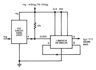
Figure 26. Voltage-to-Frequency Converter with Square-Wave Output Using ÷ 2 Flip-Flop
