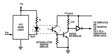
Figure 27. Voltage-to-Frequency Converter with Isolators
