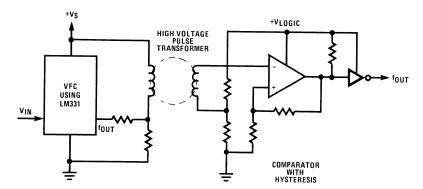
Figure 28. Voltage-to-Frequency Converter with Isolators
