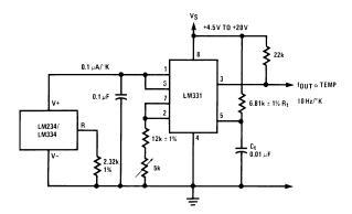
Figure 21. Temperature to Frequency Converter
