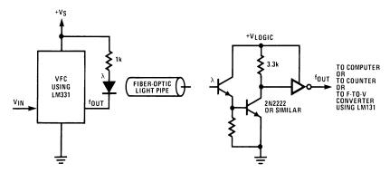
Figure 30. Voltage-to-Frequency Converter with Isolators
