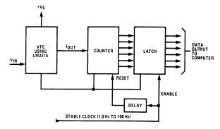
Figure 23. Basic Analog-to-Digital Converter Using Voltage-to-Frequency Converter
