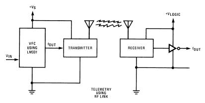
Figure 29. Voltage-to-Frequency Converter with Isolators
