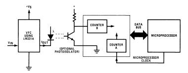
Figure 24. Analog-to-Digital Converter with Microprocessor
