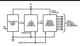
Figure 22. Long-Term Digital Integrator Using VFC
