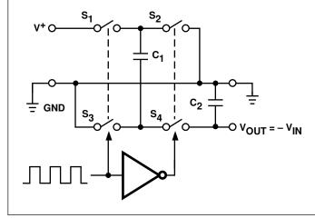
Figure 2. Idealized Charge Pump Inverter
