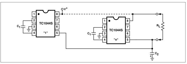
Figure 4. Paralleling Devices Lowers Output Impedance
