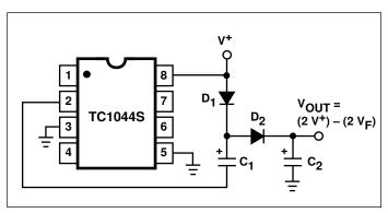
Figure 8. Positive Voltage Multiplier
