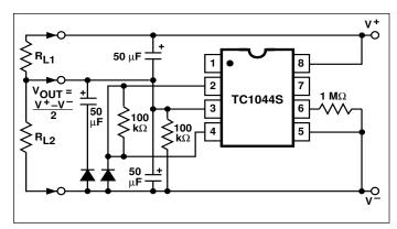
Figure 11. Splitting a Supply in Half
