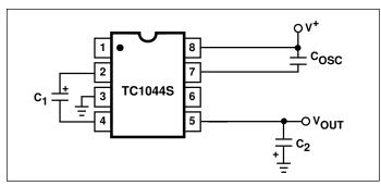
Figure 7. Lowering Oscillator Frequency
