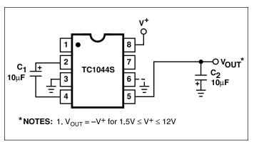
Figure 3. Simple Negative Converter
