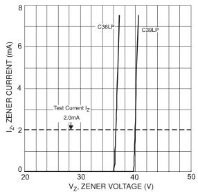
Fig. 6 Typical Zener Breakdown Characteristics
