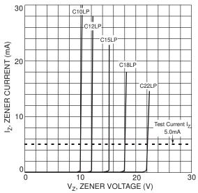
Fig. 5 Typical Zener Breakdown Characteristics
