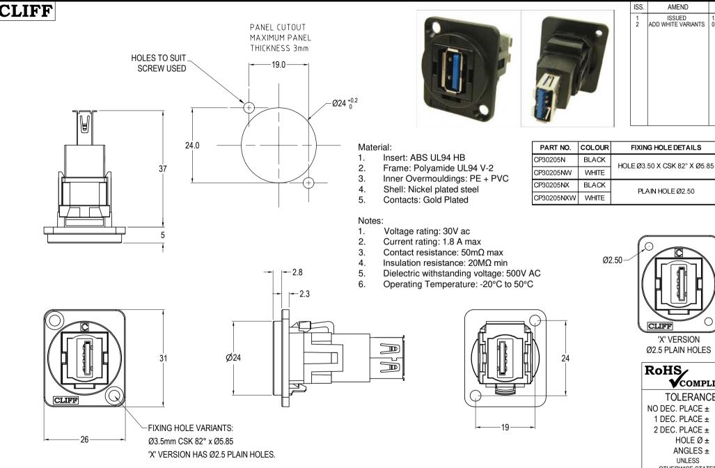
DIMENSIONS IN MILLIMETERS UNLESS OTHERWISE STATED. WORK TO DIMENSIONS. REMOVE ALL BURRS. IF IN DOUBT ASK.
