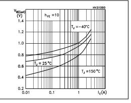
Figure 8. Base-emitter on voltage
