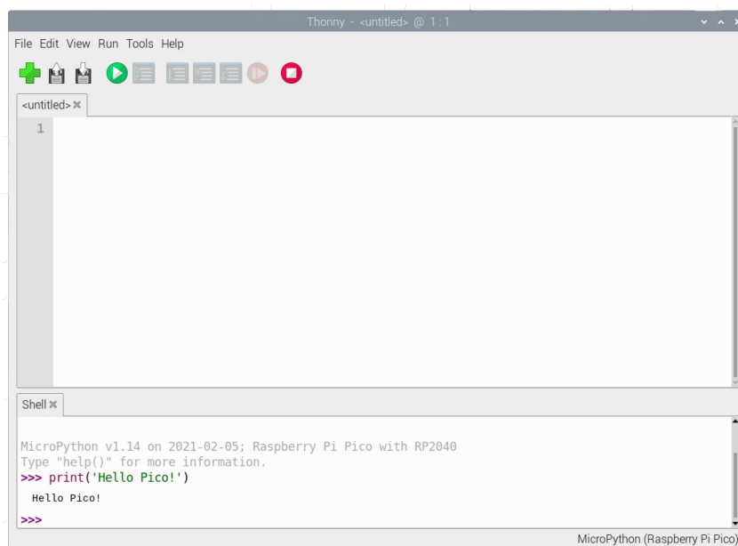
Figure 4. Saying "Hello Pico!" from the MicroPython REPL inside the Thonny environment.
