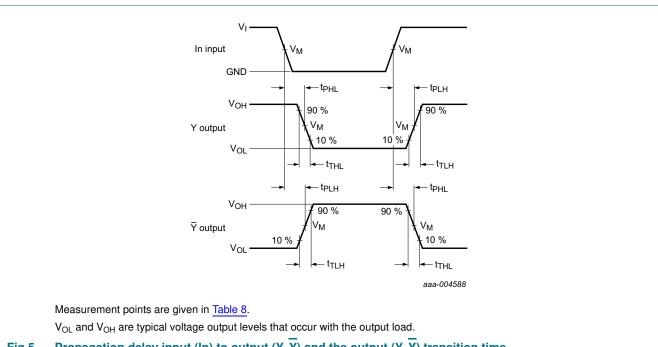
Propagation delay input (In) to output (Y, Y) and the output (Y, Y) transition time Fig 5.
