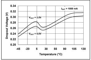
**FIGURE 2-20:** Dropout Voltage vs. Temperature.
