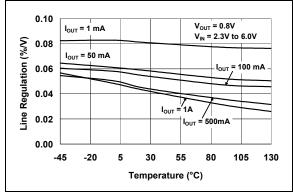
**FIGURE 2-15:** Line Regulation vs. Temperature.
