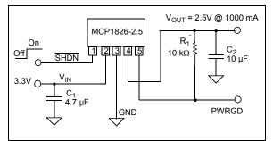
FIGURE 5-1: Typical Application Circuit.
