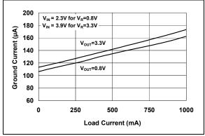
FIGURE 2-12: Ground Current vs. Load Current.
