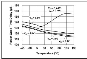
FIGURE 2-9:Power Good (PWRGD)Time Delay vs. Temperature.
