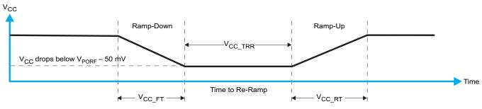
$V_{CC}$  is Lowered Below the POR Threshold, Then Ramped Back Up to  $V_{CC}$
